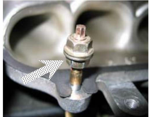
You are now ready to remove the guide pin. Use the 10mm open ended wrench on the bottom nut to unscrew it. For easy alignment, leave the two 4mm guide pins in but loosened so that they can be removed after the plenum top is lowered.
