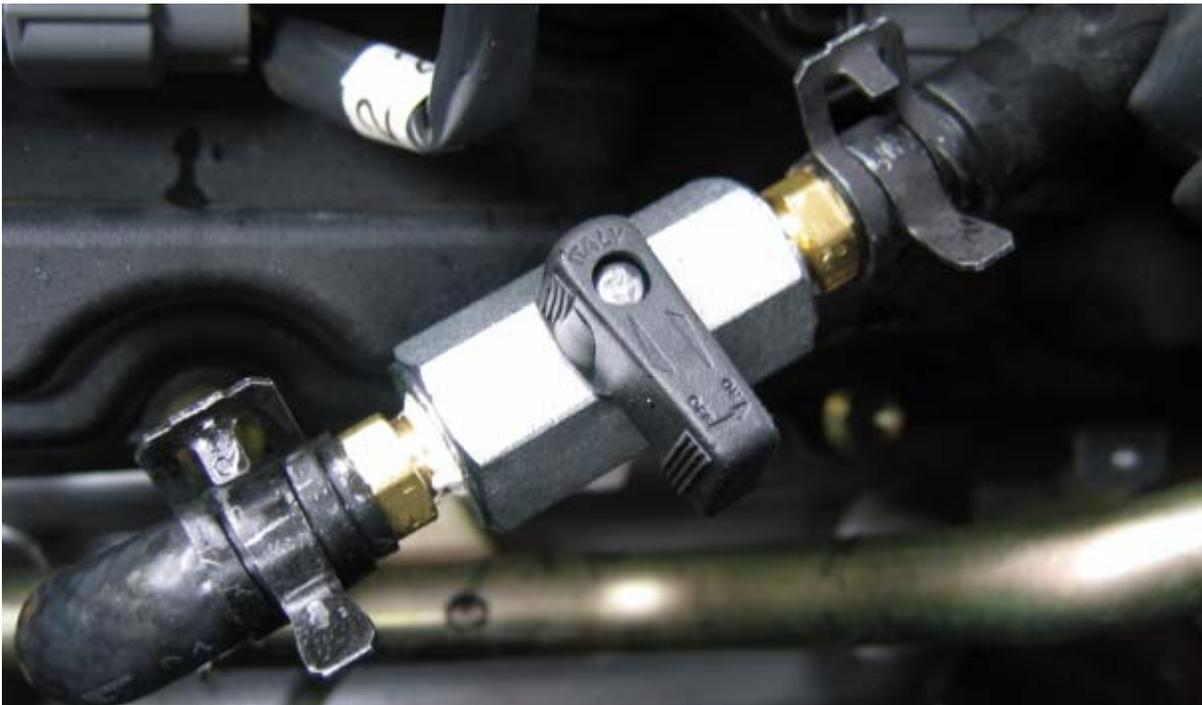
When installed the valve will be hidden under the air intake tube and will have just enough access for manual adjustment. The valve as shown above is in its closed position. The flow is shut off when the handle is perpendicular to the valve body. Conversely, it is open when the handle is parallel to the valve body. For best performance, the valve should remain closed when ambient atmospheric temperatures are above 55°F but it should always be opened at temperatures of 55°F or lower.
