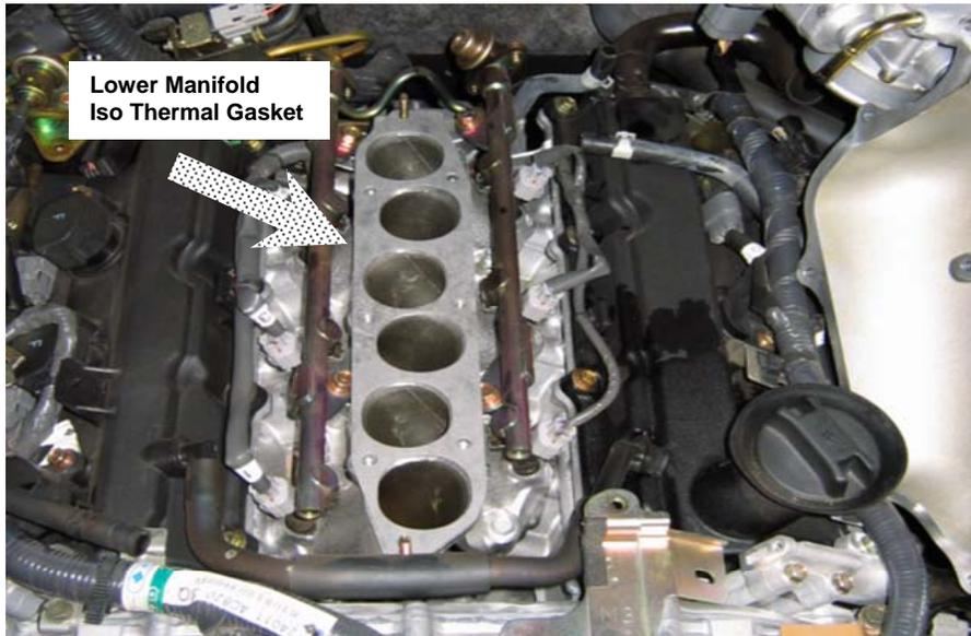
If you are installing a MREV2 first clean it of any debris or dust, then replace the old lower collector with the MREV2. Verify correct orientation of the gasket when it is placed on the intake manifold then install the lower plenum assembly.
