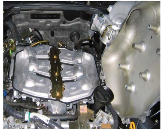
After cleaning, leave the upper plenum set it aside to allow room for removal of the lower plenum and installation of the Iso Thermal gasket. (Iso Thermal and MREV2 only)
