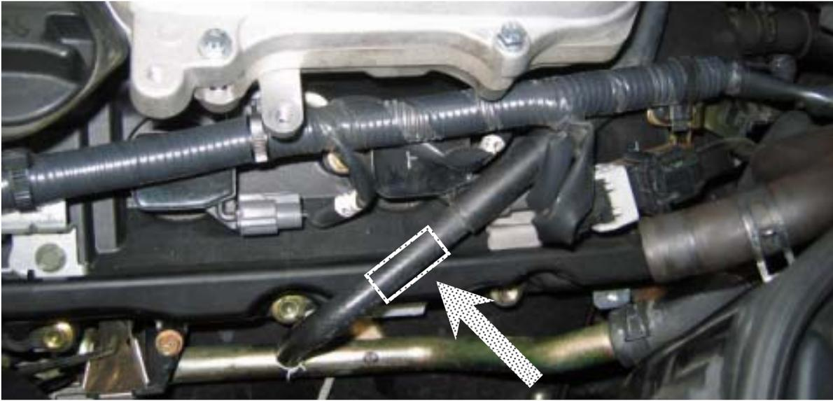
Then install the valve as shown below. The threaded fittings should be sealed with Teflon pipe thread putty or Silicone RTV for a good seal. The valve may also be painted black to reduce its visibility. The valve should be mounted facing up and slightly outward so it can be adjusted.
