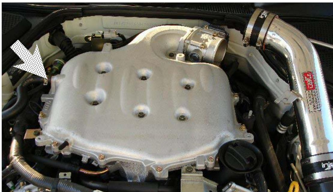
Loosen and remove all plenum bolts:
